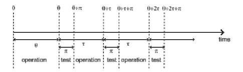
**Figure V-6.** Meaning of parameters  $\tau$ ,  $\theta$  and  $\pi$  of the "periodic-test" built-in.
