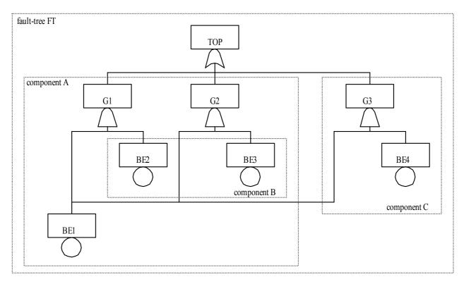
Figure IV-6. A Fault Tree with Three Components
