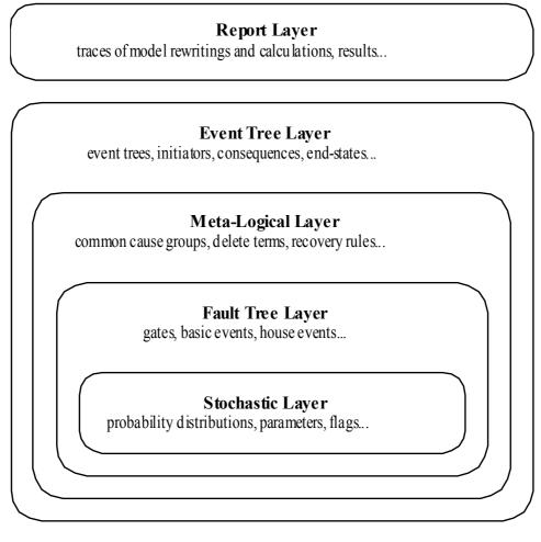
Figure II-1. Architecture of the Model Exchange Format
